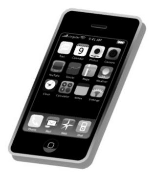
The iPhone 4 includes a panel laminated on the glass which uses electrical fields to sense the user's touch. It has a multi-touch feature that can register simultaneous touches. The user can bring up different information or menus by actions such as swiping, tapping and pinching. Information is displayed on the panel using a "Retina display".
